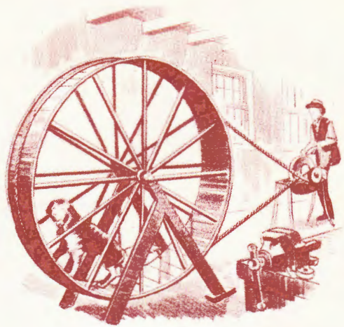
A St. Bernard dog in a treadmill supplied the power for the first Wiss grinding and polishing wheels.
